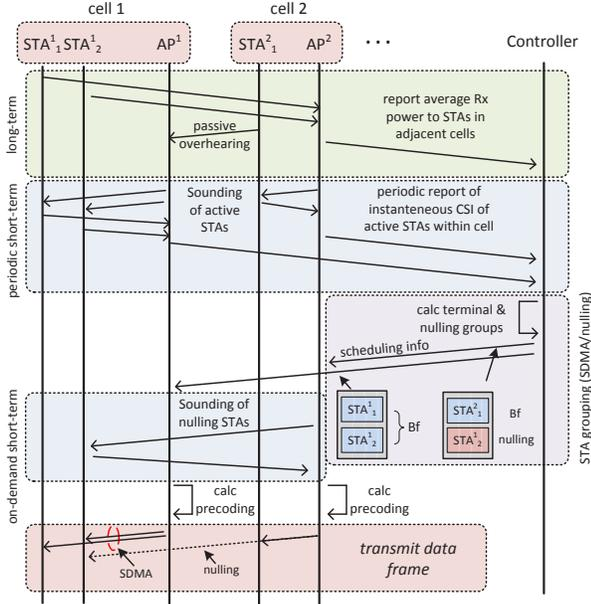
Fig. 4: Data and control flow in the proposed architecture.
