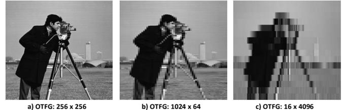
Fig. 4. Image processing (i.e. grid resampling) as the analogy of cross-technology OFDM signal reception — due to different OTFG dimensions at transmitter (a) and CTC receivers (b and c), the transmitted signal cannot be fully recovered at the receivers.
