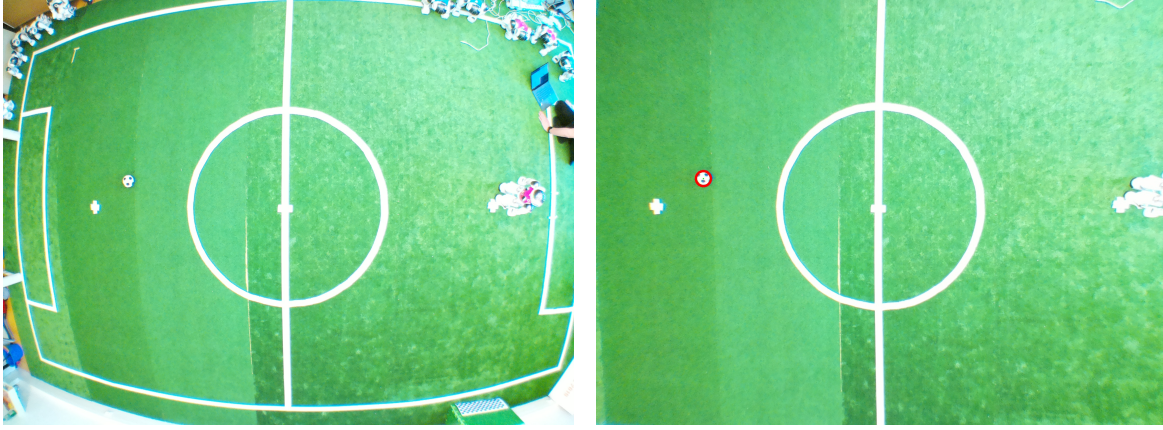
(a) Raw view of the top down camera after a kick. (b) Cropped, undistorted and automatically annotated image.
