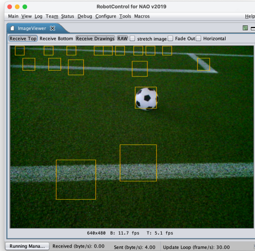
Figure 12: Visualization of ball hypothesis generation during gameplay. The image shows a recorded image log from the top camera being replayed in the RobotControl debug software, with ball candidates overlaid as yellow rectangles.
