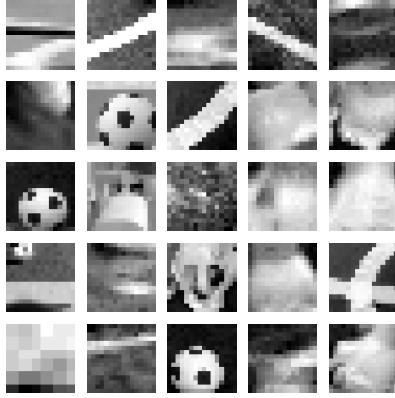
Figure 14: A random selection of 25 ball candidate image patches used for unsupervised autoencoder training. Image patches have a width and height of 16 pixels and one luminance channel (grayscale).
