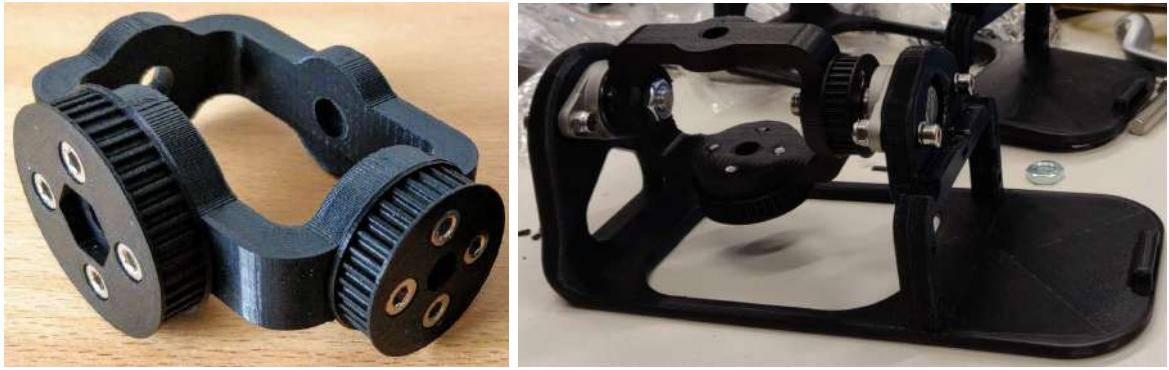
Figure 3.5: The first picture illustrates the ankle joint. This photo was taken from the assembly documentation [40]. In the left picture: the foot with the gimbal joint attached.
