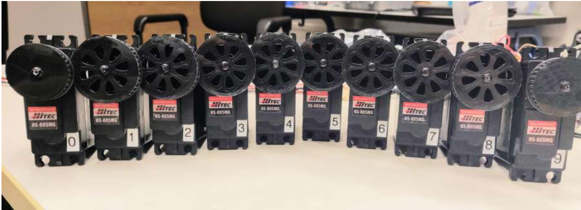
Figure 4.3: All 10 servo motors displayed, before being connected in a chain, labeled from 0 to 9.
