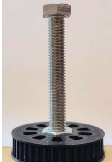
Figure 3.3: The nuts should be glued carefully into the pulleys, so that the bolts are strictly perpendicular to their surface. In this picture the bolt is slightly flexed to the left.
