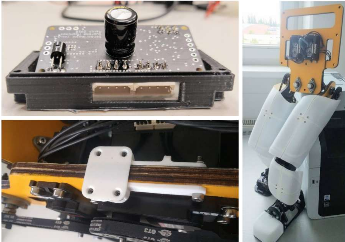
Figure 3.6: Top left picture: The Sensorimotor board situated halfway inside the 3D-printed motor cover. The side hole is slightly shifted to the right and the board doesn't fit inside the motor cover. Bottom left picture: A permanently attached adapter to the wooden part enables a quick assembly and removal of the shells. Right picture: The shells are protecting the thighs, shanks and feet of the robot. The last two pictures were taken from the assembly documentation [40].
