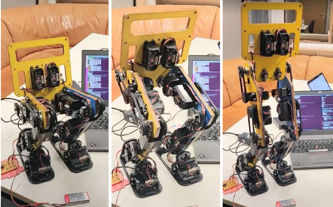
Figure 4.4: The standing up motion of the Gretchen robot, by interpolating through the sitting, squatting and standing positions
