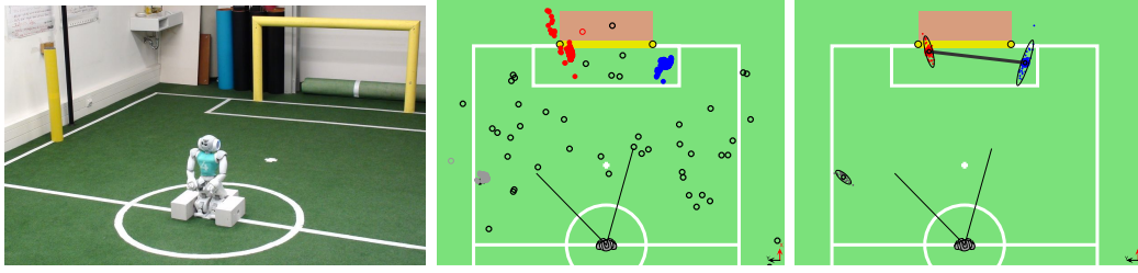
Figure 5.3: The left figure illustrates the experiment setup. The robot faces the goal and an additional goal post is placed to its left side. From the object recognition perspective, this post is identically to the real goal posts. The figure in the center visualizes all percepts collected during the course of the experiment. The full circles illustrate perceived goal posts, whereby their color indicates the classification by the MHGM: red - left post, blue - right post, gray - unknown post, black - none (percept buffer). The circles with holes stand for artificially generated sparse false positive perceptions. The right figure illustrates a snapshot of the state modeled by the MHGM at the end of the experiment. Drawn are the particle filter representing the goal posts with corresponding deviations as well as the extracted goal model. Similar to the figure in the center, the colors of the particles indicate the classification of the hypotheses.
