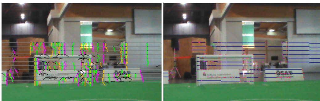
Figure 4.6: The scan lines [grey lines] above and below the estimated horizon are used to detect the goal post border points and the orientation of the corresponding edges [colored and black segments] (left). The results are features of possible goal posts [blue line segments with red dots] (right).
