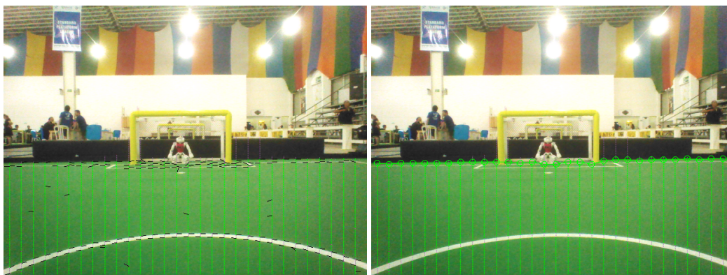
Figure 4.4: With top to down scanlines [green lines] the edges of possible field lines [black lines] including their orientation are detected (left) and the last field colored points are assumed as endpoints of the field [green circles] (right).
