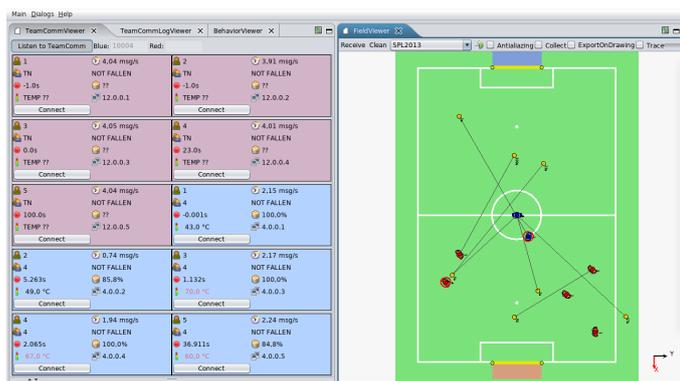
Shows all connected robots and some of their provided status information (e.g. ip address, battery charge, temperature, etc.). This dialog is mainly used during competitions to get a quick view of the robots health status. Positions of the robots, role decision and seen ball for each robot are visualized in the FieldViewer 3.2.
