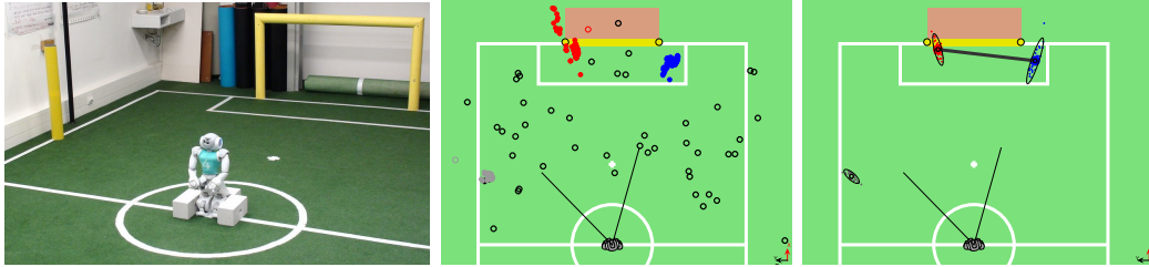
Figure 6.2: The left figure illustrates the experiment setup. The robot faces the goal and an additional goal post is placed to its right side. From the object recognition perspective, this post is identically to the real goal posts. The figure in the center visualizes all percepts collected during the course of the experiment. The full circles illustrate perceived goal posts, whereby their color indicates the classification by the MHGM: red - left post, blue - right post, gray - unknown post, black - none (percept buffer). The circles with holes stand for artificially generated sparse false positive perceptions. The right figure illustrates a snapshot of the state modeled by the MHGM at the end of the experiment. Drawn are the particle filter representing the goal posts with corresponding deviations as well as the extracted goal model. Similar to the figure in the center, the colors of the particles indicate the classification of the hypotheses.
