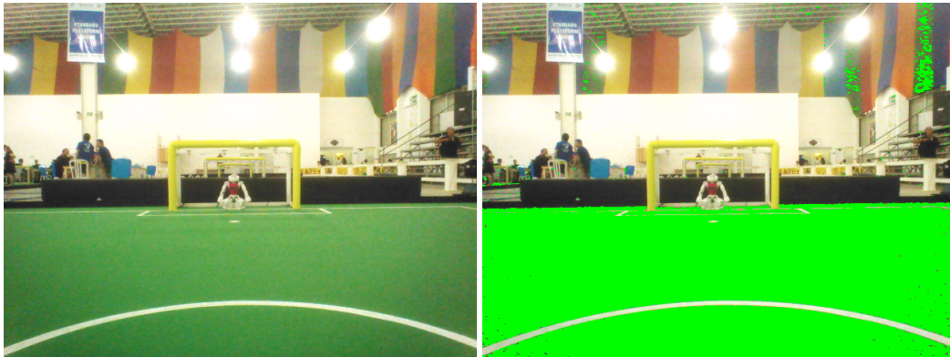
Figure 5.1: The color of the field, which is covering most of the image pixels (left), is estimated by using statistics (right).
