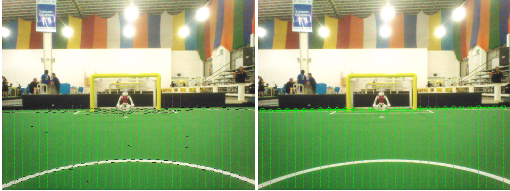
Figure 5.2: With top to down scanlines [green lines] the edges of possible field lines [black lines] including their orientation are detected (left) and the last field colored points are assumed as endpoints of the field [green circles] (right).
