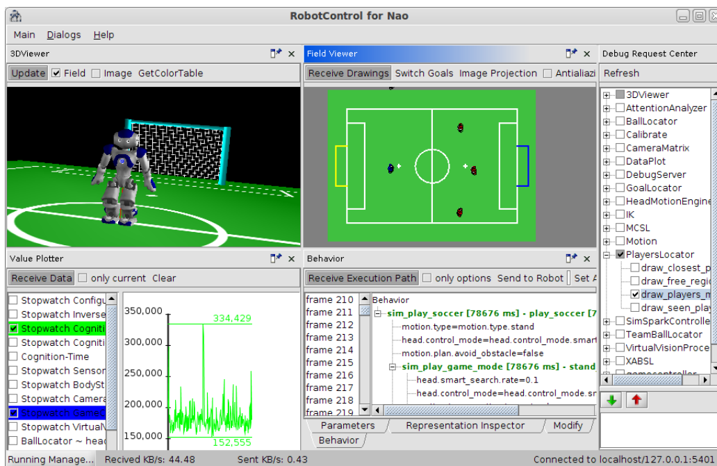
Figure 3.1: The RobotControl program contains different dialogs. The 3DViewer (top left) is used to visualize the current state of the robot; the Value Plotter dialog (bottom left) plots some data; the Field Viewer dialog (top center) draws the field view; the Behavior dialog (bottom center) shows the behavior tree; the Debug Request Center dialog (right) is for enabling/disabling debug requests.
