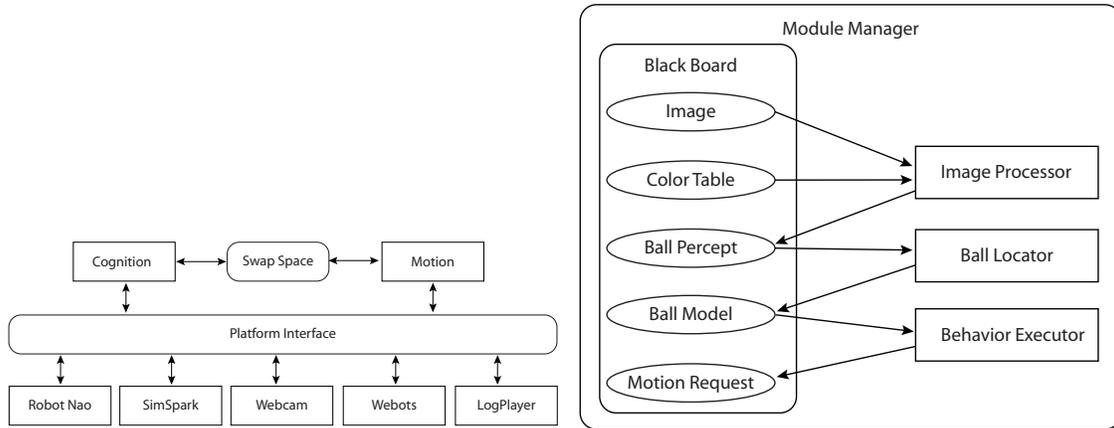
**Fig. 1.** Schematic illustration of the *platform interface* (left) and the *module architecture* (right).
