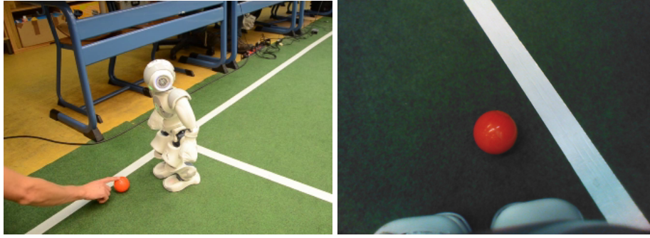
Fig. 1. The left figure shows an example scenario where the robot observes a ball in front of a line. The figure on the right shows the situation from the perspective of the robot’s camera.
