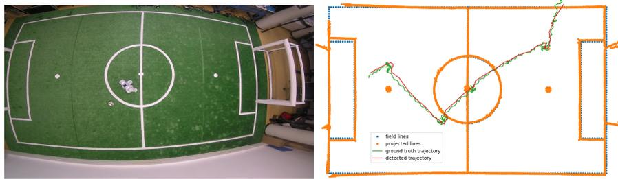
**Fig. 6.** Tracking of the robot in the laboratory conditions. Left: a frame from the recorded video. Right: trajectory of the robot determined based on the video in comparison to the ground truth recorded by the OptiTrack system. Projected line points are also shown in comparison to the model of the field. Note the goal posts being treated as lines.
