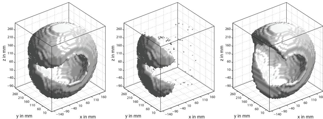
Figure 2. The *reachable space* of the Nao's hand is approximated by a three dimensional grid; (left) the theoretical reachable grid generated in simulation; (right) reachable positions with the fixed yaw-joint in the elbow; (center) difference between both grids;
