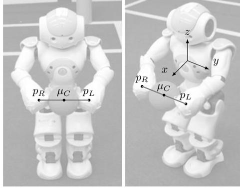
Figure 3. Geometry of the grasping motion:  $\mu_C$  denote the center of the grasping motion (e.g., estimated center of gravity of the ball),  $p_L$  and  $p_R$  are the desired points for the hands.
