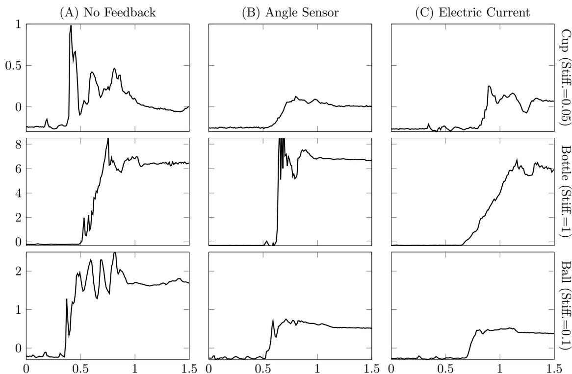
Figure 5. Force measured at the end effectors during the grasping of three different objects using different controllers as described in Section 4.2 with a fixed stiffness for each object.
