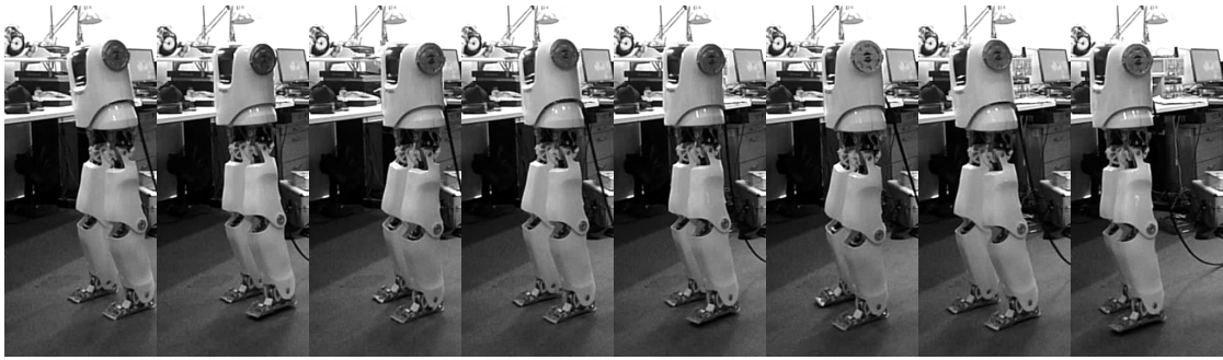
Figure 1.20: The Myon robot’s trunk with legs while walking small steps: A penguin-like gait pattern, similar to toddling, emerges from reconstructing a periodic (or clock) signal from sensory data and feeding it back to the leg motors with individual phase and amplitude. The created dynamical system exhibits co-existing attractors, such as a fixed point for standing and a quasi-periodic orbit for toddling. An intended laterally applied nudge suffices to leave the equilibrium and enter the basin of the stable gait pattern’s attractor. Vice versa, gently holding the robot stops the oscillation again.
