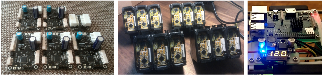
Figure 8.11: Electronic components installed into the robot: 5 Limbcontrollers, 1 power distribution node, 12 Sensorimotors, and a Raspberry Pi 4 using a separate 5V voltage regulator.
