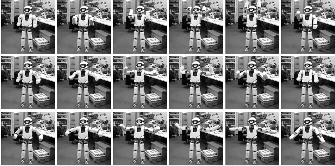
Figure 1.12: Example 3) Sequence of gestures using CSLs. Arms are raised using contraction mode and taken down using release mode. The CSLs for shoulder pitch/roll and elbow joints are activated according to the position of the other joints in order to create different contraction/release sequences. The execution speed of each gesture sequence can be modulated by different contraction strength and even halted at any time using hold mode. Since the angular momentum generated by the moving arms would easily make the robot fall over, CSL-driven joints are used concurrently to stabilize the torso and legs as already described in Figure 1.11.
