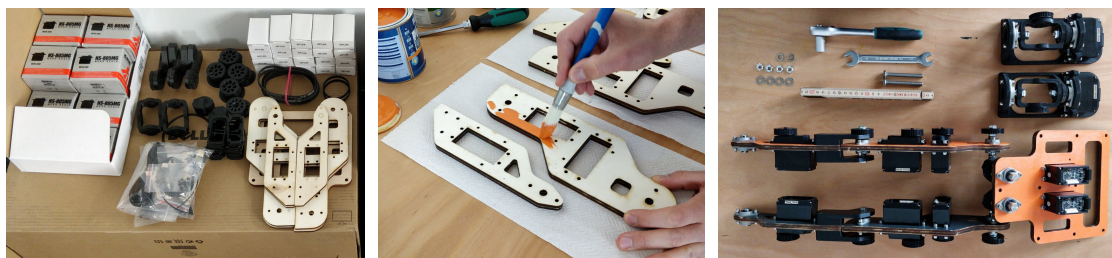
Figure 8.23: The Gretchen robot as a kit, during coloring of plywood parts, and during assembly.
