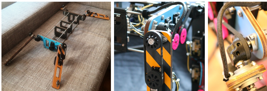
Figure 8.7: Torso during assembly and shoulder joint from different views.
