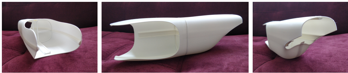
Figure 8.8: Robot shells made from 3D-printed Tough-PLA for protection of the leg electronics and belt drive. Assembling shell parts comes without tools because they possess a mechanical snap lock at their edges, connecting the shell halves solidly.
