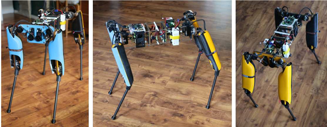
Figure 8.10: Different views on the fully-assembled robot, including shells. In the moment of these pictures, for the first time, the robot is autonomously powered by its batteries and actively maintains its balance by control loops calculated on the robot.
