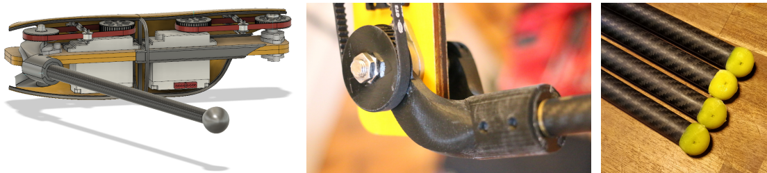
Figure 8.6: CAD model inside view of a leg with, belts, pulleys, shells and Sensorimotors (left). A detailed view on the knee (center) and silicone-cast feet (right).
