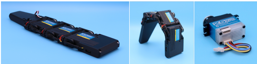
Figure 9.3: The flatcat robot undressed and a single Sensorimotor servo drive.
