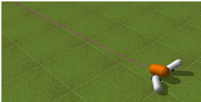
Figure 5.13: Tadpole robot crawling backward and forward learned in the fully unsupervised learning with growing states and actions: The behaviors learned in this experiment achieved approximately 50% of the performance observed in evolution experiments but required significantly less computation time (approximately 10%). While it may take the robot more time to enter the crawling attractor, the learned behaviors have the ability to switch to different behaviors mostly without getting stuck since they are learned together and share the same states and action elements. The magenta trajectory of the body clearly shows that the motion is much more irregular compared to the results from evolution shown below.
