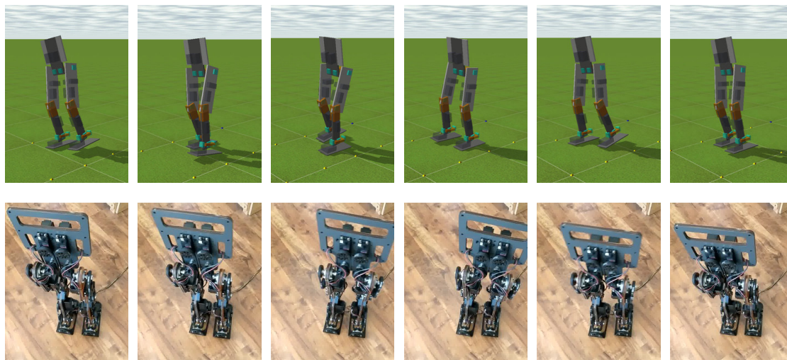
Figure 8.24: The Gretchen robot forward walking in simulation and backwards in reality.
