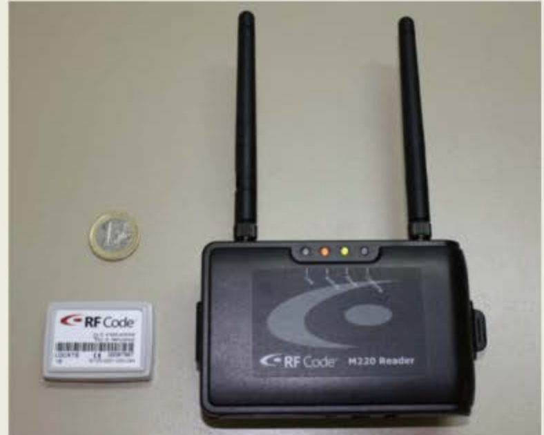
Active RFID Tag and Reader, Seco et al. (2010)
