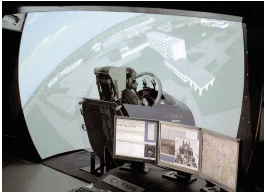
L-159B Full Mission Simulator uses latest commercial components in order to provide affordable operation and long-term supportability
