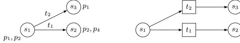
Fig. 1. Transformation from automaton to Petri net
