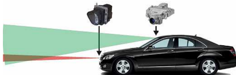
Fig. 7: Test vehicle with serial Night View Assist camera and multi-beam lidar sensor.
