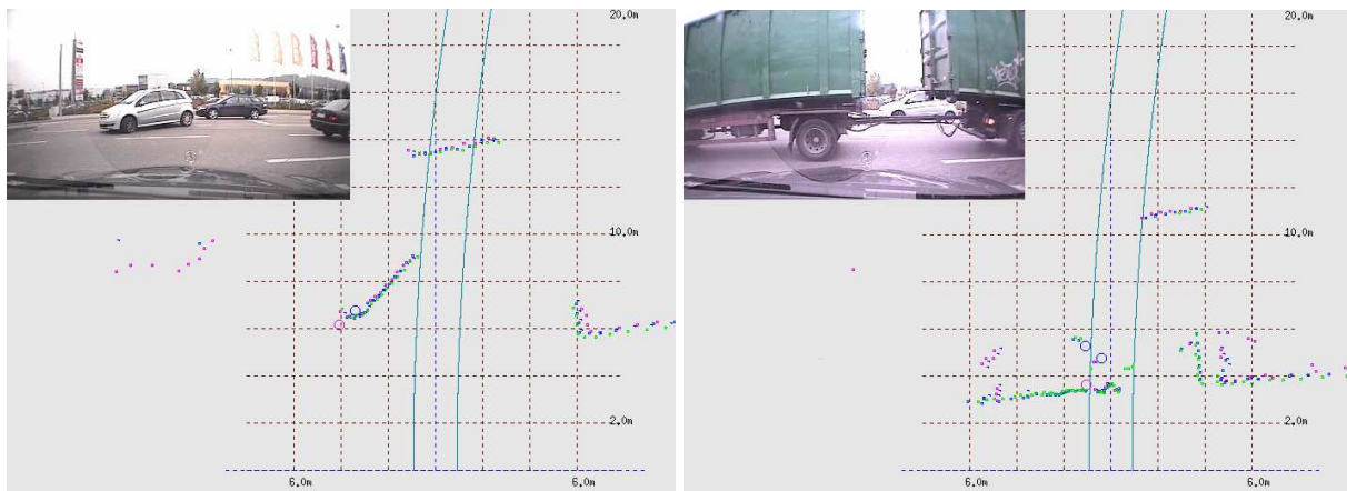
Figure 3: Environmental scan examples. Single laser echos are shown as points, the bigger circles represent radar targets.
