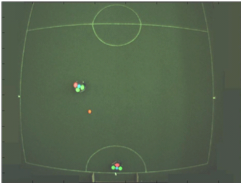
Fig. 2. Barrel distortion of the field with a 4.2 mm lens
